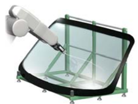
Curvature measurement of glass surface
