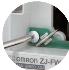
Easy electrode needle replacement
