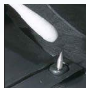
Cleaning the discharger electrodes
