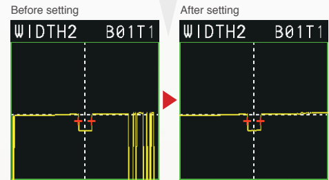
Lost part on a profile due to insufficient amount of light received
