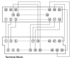
Note: Connector pin numbers correspond 1-to-1 to terminal block numbers on all models.
