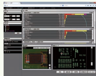
• Analysis function Shows real faults and false alarms in Pareto chart
