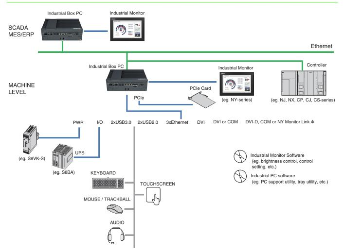
\*NY Monitor Link option: Connect monitor up to 100 m via standard Ethernet cable.
