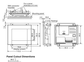
Applicable panel thickness : 1.6 mm to 4.8 mm
