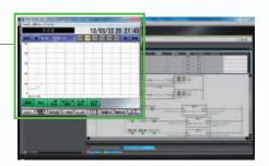
Test screen of CX-Designer appears after synchronization of Sysmac Studio, and integrated simulation starts.
