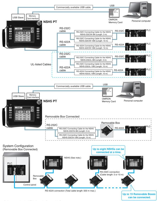
Note: Before removing the NSH5 from the Removable Box, be sure to first turn OFF the power supply key on the Removable Box.
