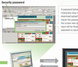
A password between 4 and 64 characters long can be set. The download/upload will start if the user inputs the password that was set when the screen was designed. (Password input will be disabled if the wrong password is input 3 times in a row.)
