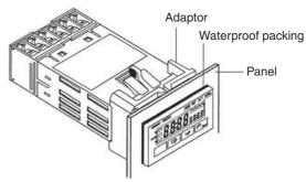
The H8GN's panel surface is water-resistive (conforming to NEMA 4X (indoors) and IP66). In order to prevent the internal circuit from water penetration through the space between the Counter and operating panel, attach a rubber packing (provided with the H8GN) between the Counter and operating panel and secure the rubber packing with the Flush-mounting Adaptor.
