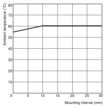
Testing Method Tested Timer: H3DT-A Applied voltage: 240 VAC Installation pitch: 0 and 10 mm
