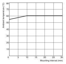
Testing Method Tested Timer: H3DT-H Applied voltage: 240 VAC Installation pitch: 0 and 10 mm Load current: 5 A
