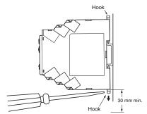
It will be easier to mount and dismount the Timer if a distance of 30 mm or more is provided between the bottom of the Timer and other equipment.
