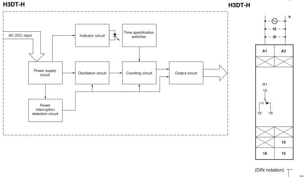
Note: The above figure shows the terminal arrangement for a 24 to 48-VAC/DC model. Models with 100 to 120-VAC or 200 to 240-VAC power input do not have a DC input. \* The power supply terminals do not have polarity.
