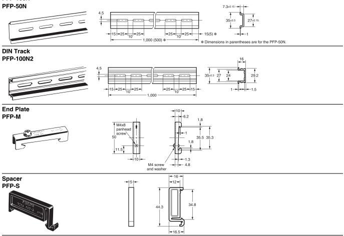
Note: 1. Order the above products in multiples of 10.2. The Tracks conform to DIN standards.
