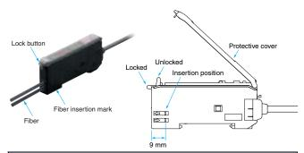
Note: Do not pull on, compress, or otherwise exert excessive force on the fibers after connecting them to the Amplifier Unit.
