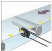
Through-beam Fiber Heads are capable of detecting color differences in semi-transparent objects.
