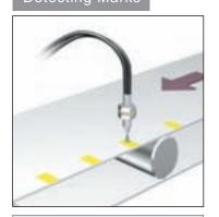
Because it distinguishes RGB ratios, detection is highly resistant to workpiece movement.
