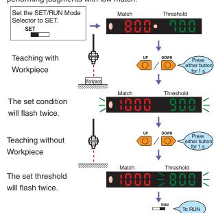
\* When teaching is performed, position the workpiece by using the OVER, OK, and LO messages displayed on the sub-display (green) as guides.
