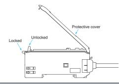
Note: 1. To maintain the fiber unit properties, confirm that the lock is released before removing the fiber units.
