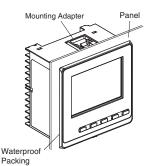
In order to make the unit waterproof, with the accessory waterproof packing on the front of the panel, insert the unit into the panel opening. Unless the waterproof packing is put, the product is not
