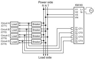
Single-phase, Three-wire Circuit and Single-phase, Two-wire Circuit Branched from Single-phase, Three-wire Circuit
