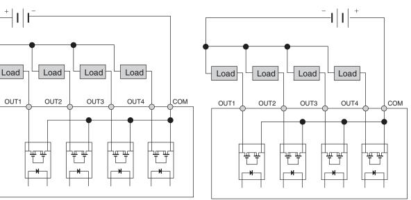
The Power Monitor provides four pulse output terminals. One common is used.
