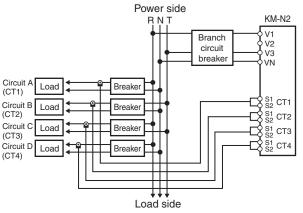
Single-phase, Three-wire Circuit and Single-phase, Two-wire Circuit Branched from Single-phase, Three-wire Circuit
