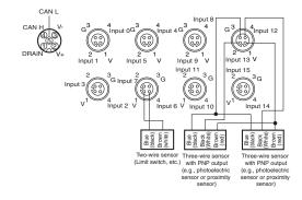
**Environment-resistive Terminals with Transistors (Standard Type)**
