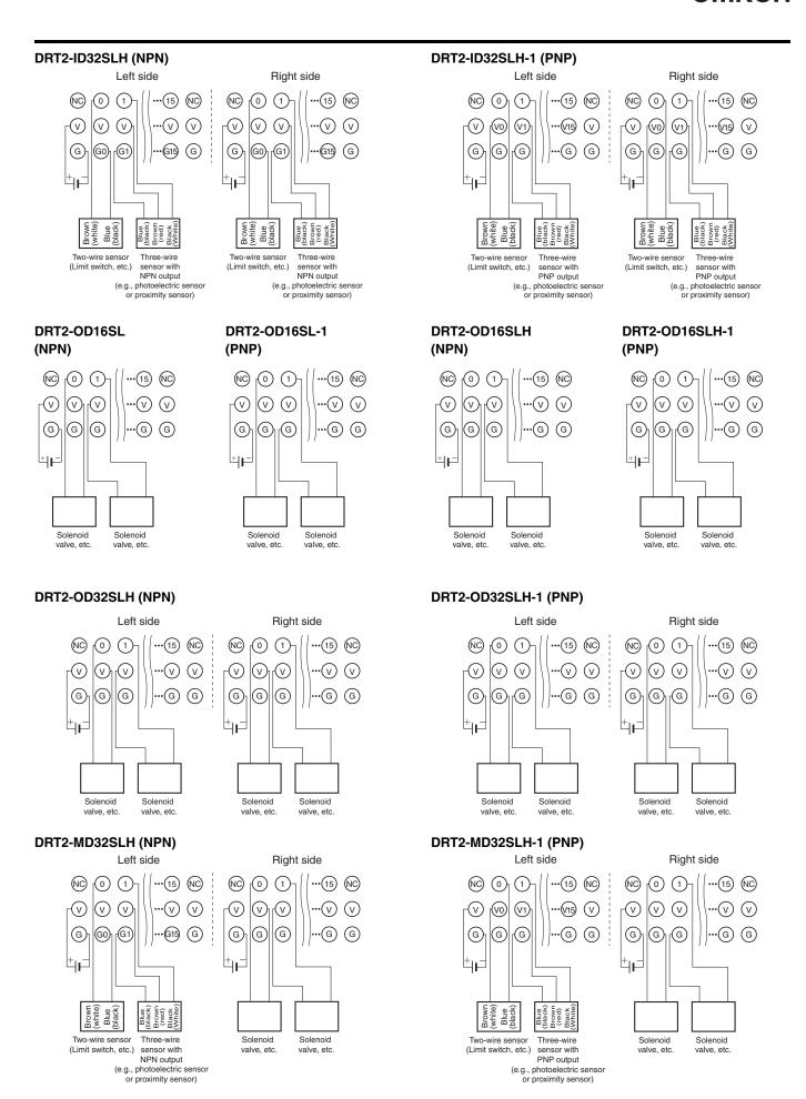
**Environment-resistive Terminals with Transistors (High-function Type)**
