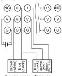
Two-wire sensor Three-wire sensor with PNP output (e.g., photoelectric sensor or proximity sensor)
