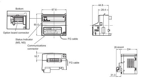
After the DeviceNet Communication Unit is installed, dimension D of the inverter increases by 26.4 mm (Dimension D of the inverter varies depending on the capacity. Refer to the MX2-series USER'S MANUAL (Cat.No.I585)) High-function General-purpose Inverters RX-Series V1 type DeviceNet Communication Unit
