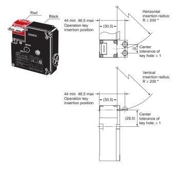
D4NL + D4DS-K1 (with Top-inserted Operation Key)
