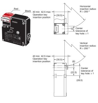
D4NL + D4DS-K2 (with Top-inserted Operation Key)
